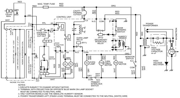
Figure O-2. Oven Schematic-Cooking Condition
